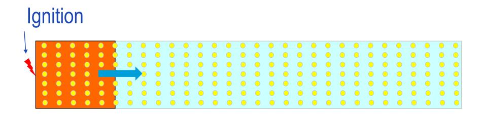
Maximises flow through pipes giving rapid flame acceleration
